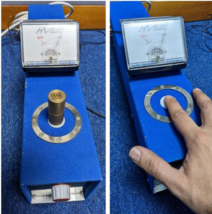
Figure 9. The HV Lab tactile vibrometer for measuring the thresholds was calibrated with 2 N weights before measuring vibrotactile thresholds.
