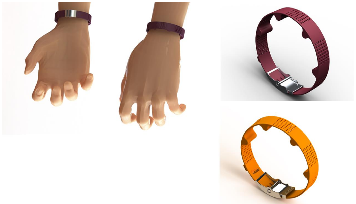
Figure 32. A prototype for a wrist-worn haptic device based on the MosaicOne_C design is being developed by the Electro-Haptics project at the University of Southampton (Fletcher and Verschuur, 2021).
